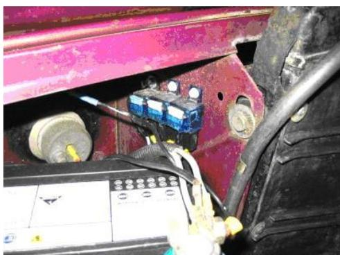
I used Hella relays incorporating a blade fuse to simplify the wiring, and negating the need for inline fuse holders. Utilising a connector with the same three male connectors as a headlamp I could use the original power to the headlamps to control the relays.
