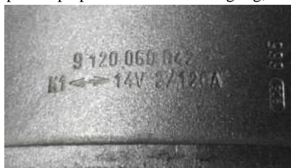
I discovered all Bosch alternators have a 10-digit number followed by more numbers letters and symbols. These specify the catalogue number as well as the physical characteristics, such as physical size, voltage, power output through rotational speed ranges, max current, and cut in speed.
